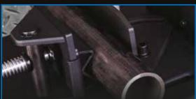
V-Block Clamp Included for Round Tube, Box Section
